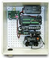
ESS Remote Processing Unit (RPU) with battery-backed power supply and phone modem
