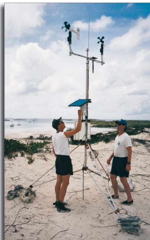
A weather station network on the Bahamas provides data for studying how weather patterns affect the transport of three marine species.
